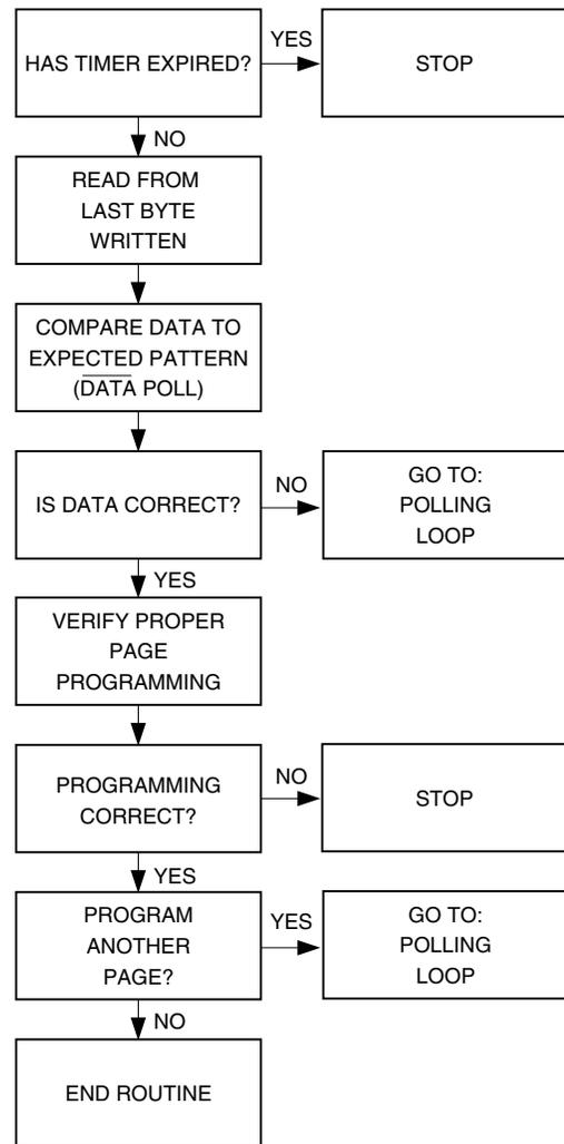
**Figure 5.** Timing Sequence for Protected Sector Write (AT29C010A 1M-bit Example)
