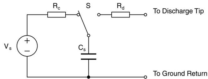
A simple way of modeling this phenomena is to use a capacitor that will hold the same charge as the body and a series resistor that will release this charge the same way the body does.
