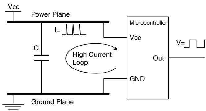
Figure 4 shows an example of insufficient decoupling. The capacitor is placed too far away from the microcontroller, creating a large high current loop. The power and ground planes here are parts of the high current loop. As a result of this, noise is spread more
