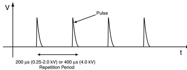
Figure 2 shows the fast transient burst pulse train used for EMC testing. Figure 3 shows a close-up of a burst. Note that the pulse is only about 50 ns wide, this is much smaller than the figure indicates. See IEC 1000-4-4 for details of the pulses and the test setup.
