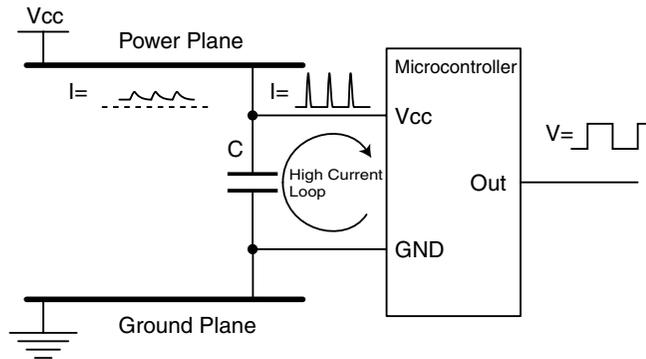
Figure 5 shows a better placement of the capacitor. The lines that are part of the high current loop are not part of the power or ground planes. This is important, as the power and ground planes otherwise will spread a lot of noise.
