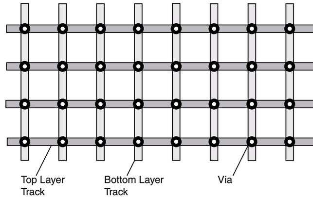
One way of designing a ground plane on a two-layer board and still allow routing on both layers, is to design a ground grid as shown in Figure 7. Here every path will have a ground return nearby, creating a relatively small loop. How large the cells and how wide the tracks should be will depend on the application. Higher currents and higher frequencies will require wider tracks and smaller cells.
