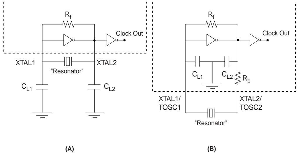
Note: 1. (A) Represents the Oscillator Circuit for Crystals and Ceramic Resonators Faster than 400 kHz, while (B) is for Low Frequency Crystals (32.768 kHz).
