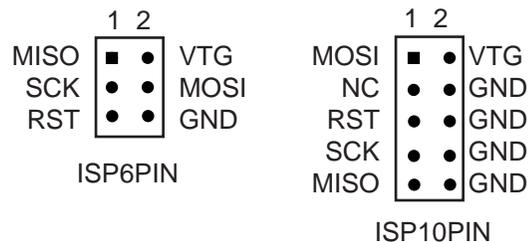
Some ISP programmers are supplied by the target power supply. In this way they easily adapt to the correct voltage level of the target board. Other ISP programmers, like STK500, can power the target board via the VTG line. In that case it is important that the power supply on the target is not switched on. Read the user guide of the ISP Programmer to find out what capabilities your programmer has and what kind of physical interface it has.
