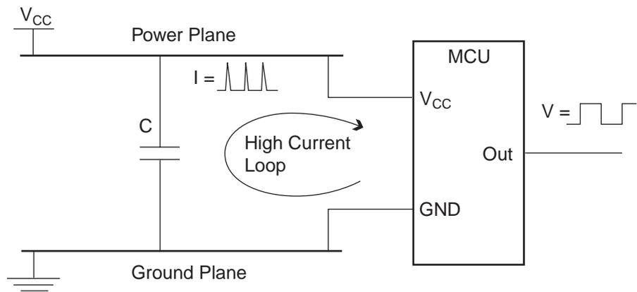
Note: 1. Decoupling Capacitor is too far away from the device.
