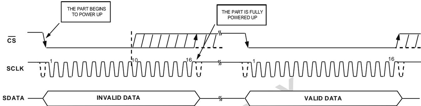
Figure 4. Exiting Partial Power-Down Mode
