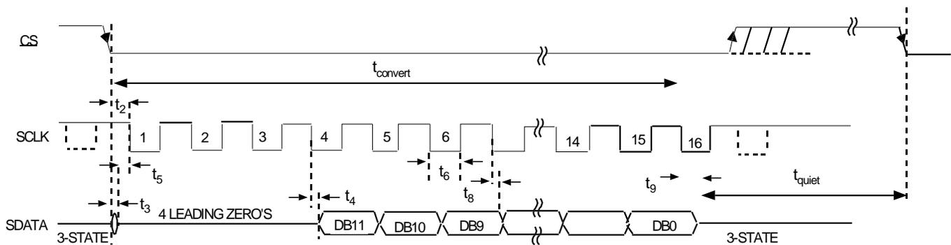
Figure 7. Serial Interface Timing Diagram
