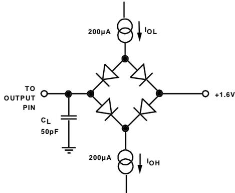
Figure 1. Load Circuit for Digital Output Timing Specifications
