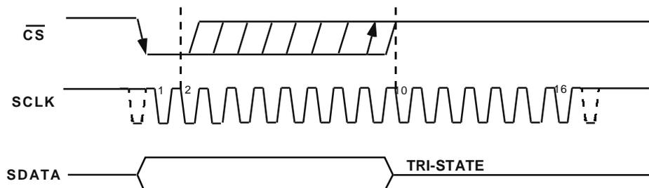
Figure 3. Entering Partial Power-Down Mode
