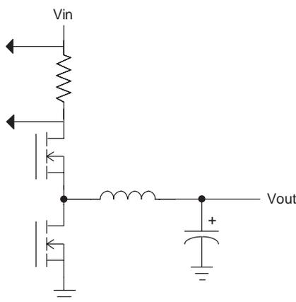
**Figure 4. Using an Input Current Sense Resistor (Conceptual)**
