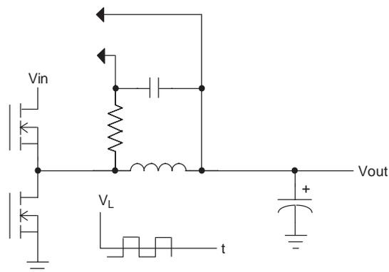
**Figure 3. Sensing the Current by Measuring the Voltage Across the Inductor Involves Filtering the Signal Because the Inductor has a Switching Waveform Applied**
