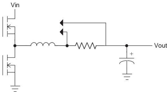
Figure 1. Using an Output Current Sense Resistor
