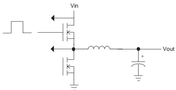
Figure 2. Sensing the Current by Measuring the MOSFET's  $V_{DS}$  Requires a Blanking Time
