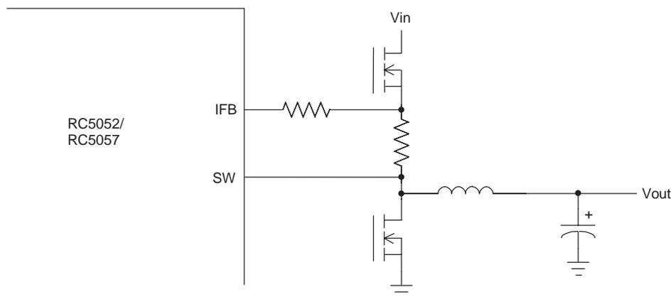
**Figure 5. Implementation of an Input Current Sensing Resistor using Fairchild's RC5052/RC5057**
