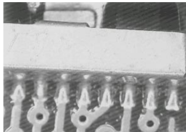
Photo 4.0. Unit self-aligns after reflow.
