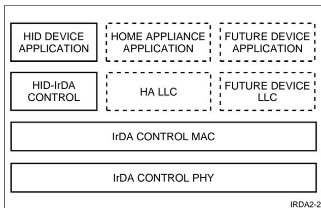
**Figure 2. System Architecture**
