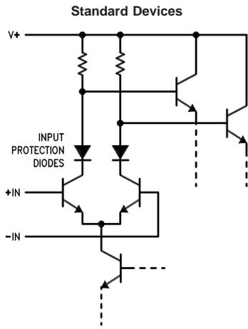
The input protection diodes are useful in certain party-line systems which may have multiple  $V+$  power supplies and, in which case, may be operated with some of the  $V+$  supplies turned off. In such a system, if a supply is turned off and allowed to go to ground, the equivalent input circuit connected to that supply would be as follows:
