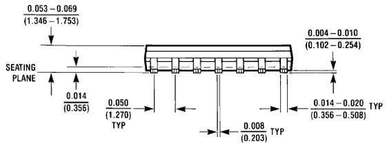
**Molded Dual-In-Line Package (M)**
