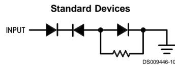
This would be a problem in specific systems which might possibly have the transmission lines biased to some potential greater than 1.4V. Since this is not a widespread application problem, both the "A" and standard devices will be available. The ratings and characteristic specifications of the "A" devices are the same as those of the standard devices.
