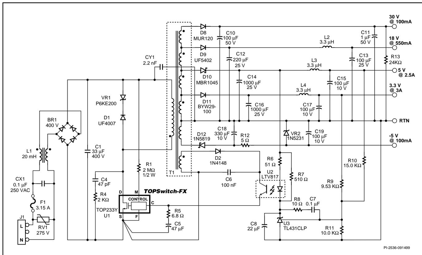
Figure 25. 35 W Set-Top Box Power Supply.
