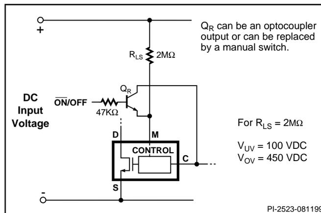
Figure 23. Active-off Remote ON/OFF with Line Sense.
