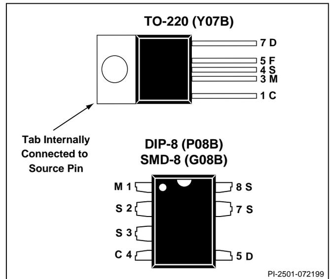
Figure 3. Pin Configuration.
