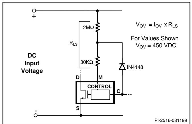
Figure 16. Line Sensing for Over-Voltage Only (Under-Voltage Disabled).
