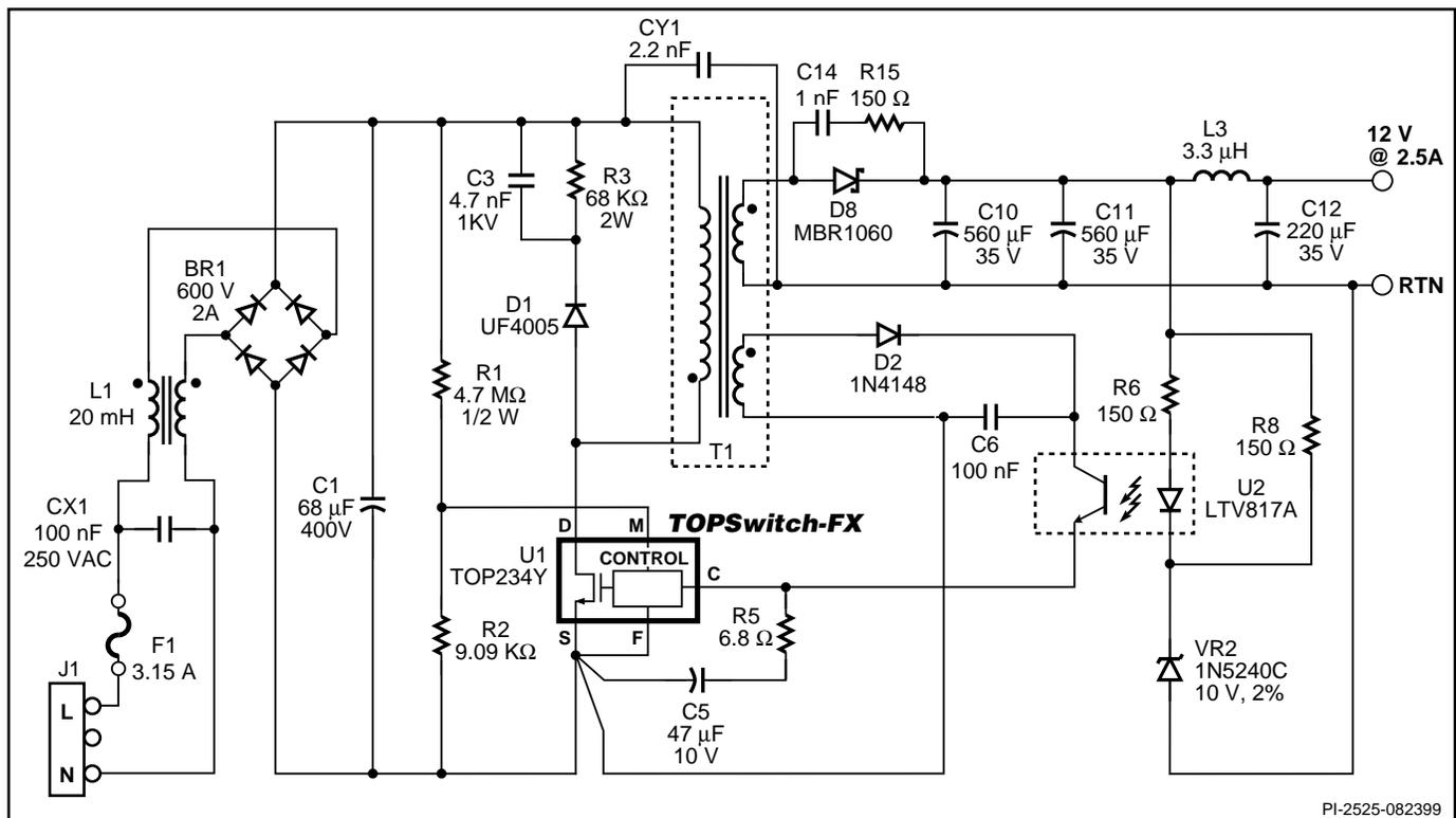
Figure 24. 30 W Power Supply using External Current Limit.
