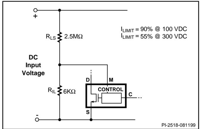
Figure 18. Current Limit Reduction with Line Voltage.
