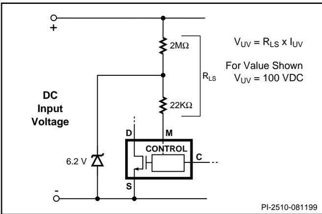
Figure 15. Line Sensing for Under-Voltage Only (Over-Voltage Disabled).
